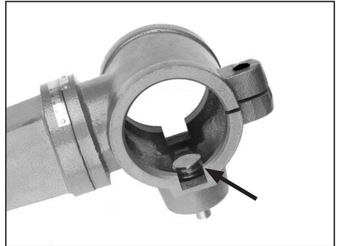
Figure 7. Pinion correctly installed in table support.
